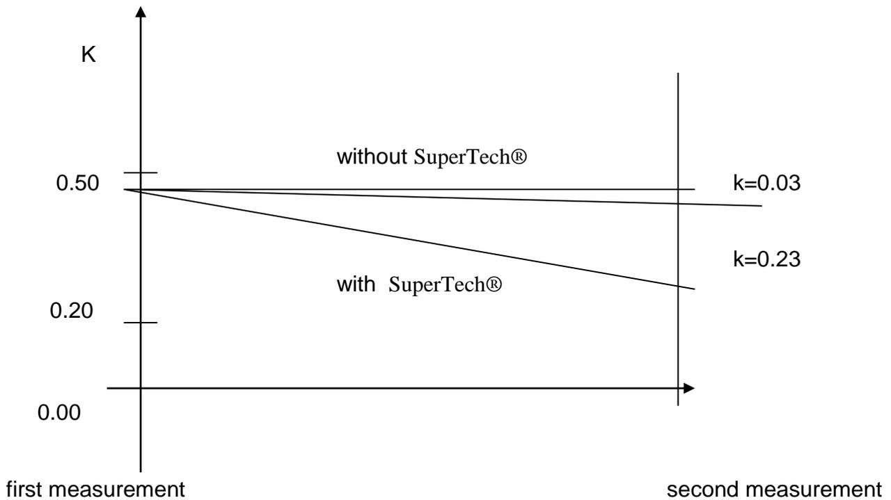
Average value of the opacity K for the first series of measurements (before the installation) Supertech result 0.45.
